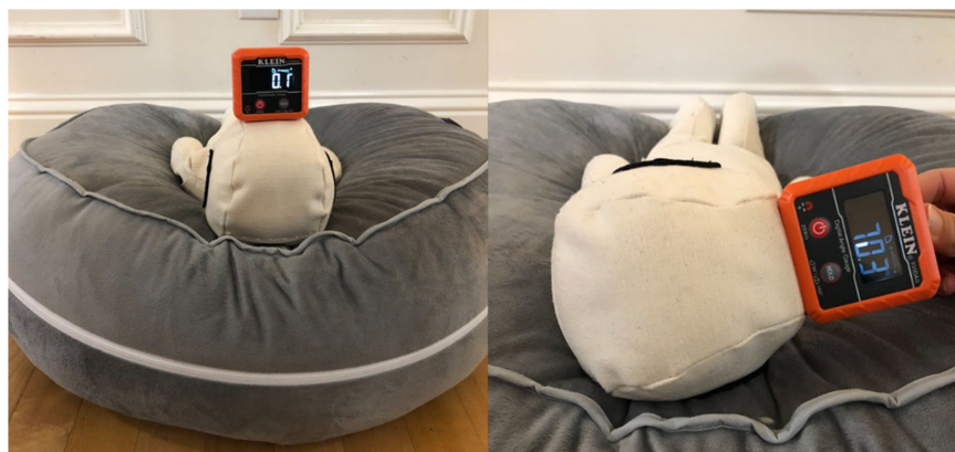
Figure 12. Photos from testing of the head rotation required during prone lying to free the mouth/nose region of the CAMI dummy to allow for free airflow.
